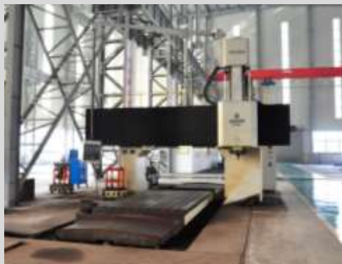
5m数控龙门钻铣床 1台 5m CNC Gantry Drilling and Milling Machine 1set
